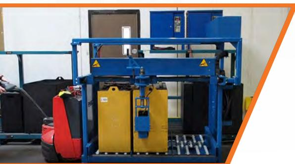
Mounts easily to powered pallet truck with 60" (1524 mm) or longer forks
